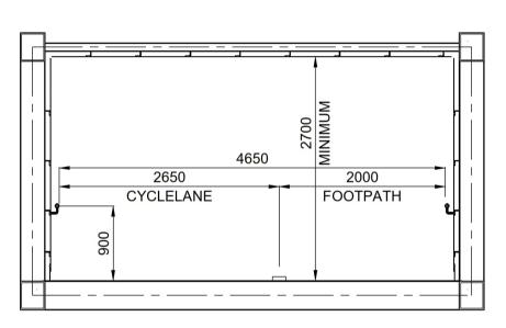
TYPICAL SECTION THROUGH ARTERIAL LINK SPAN 1:50 @ A1 1:100 @ A3
