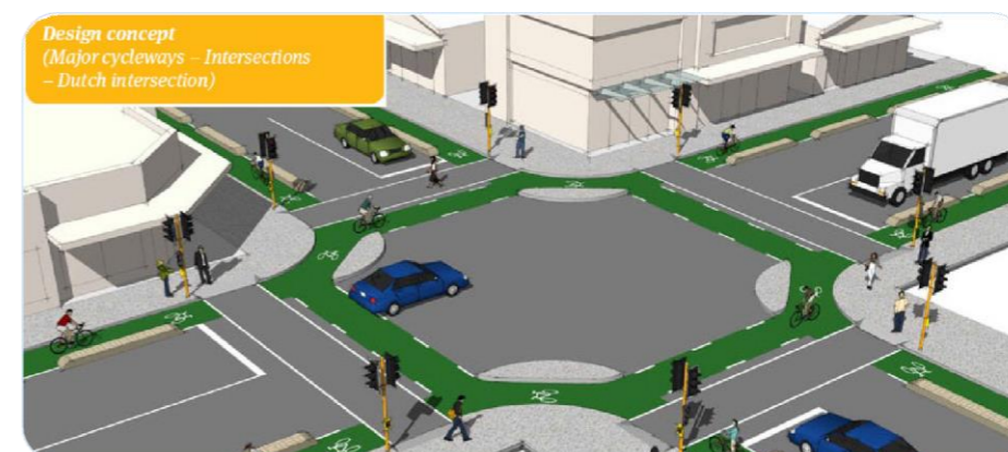
Figure 16: Key Infrastructure Elements of Protected Junction
