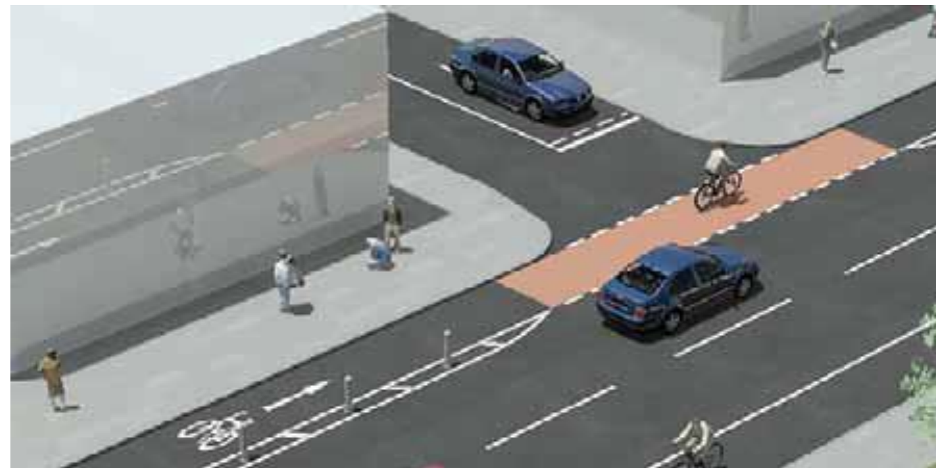
Figure 32: On-Road Cycle Lane Priority Junction Treatment
