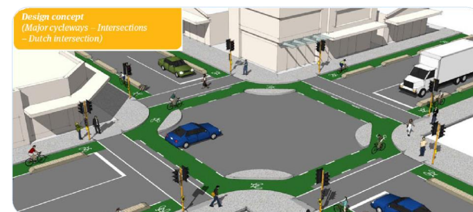
Figure 16: Key Infrastructure Elements of Protected Junction
