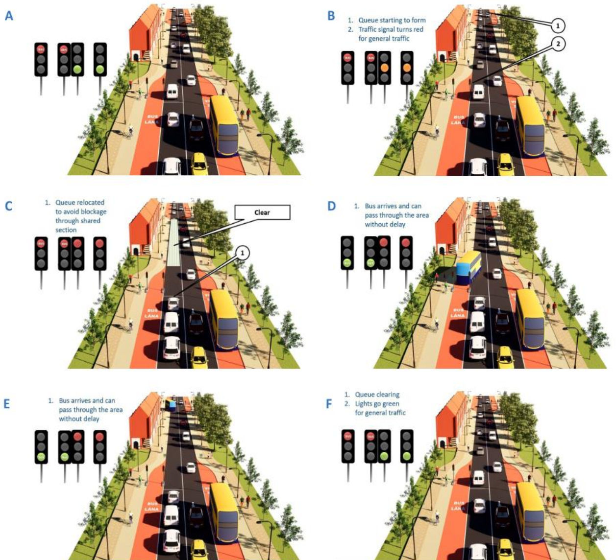
Image 4.15: Signal Controlled Priority Schematic Operation (Source: PDGB)
