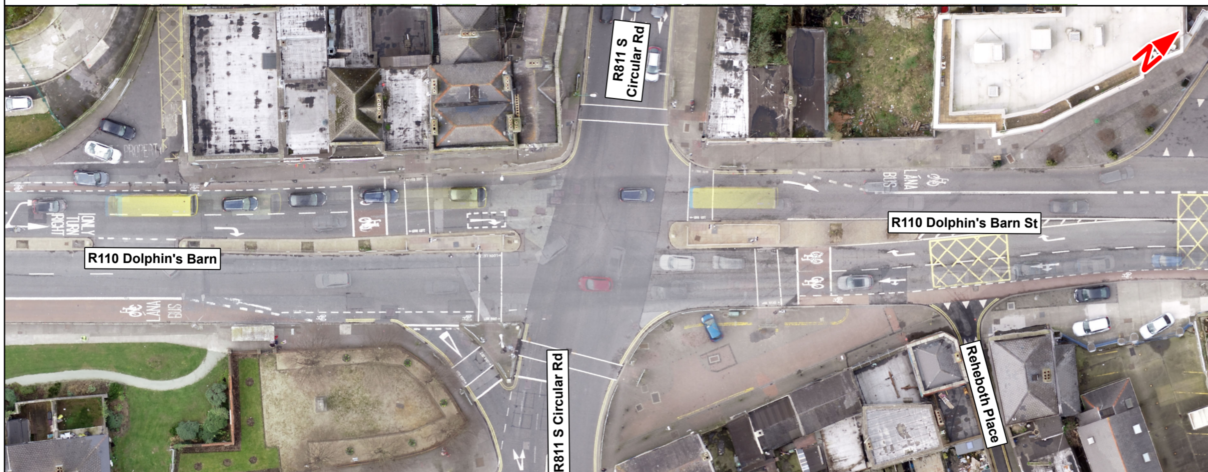
B) R110 DOLPHIN'S BARN STREET, R811 SOUTH CIRCULAR BOAD FOUR-ARM SIGNALISED JUNCTION
