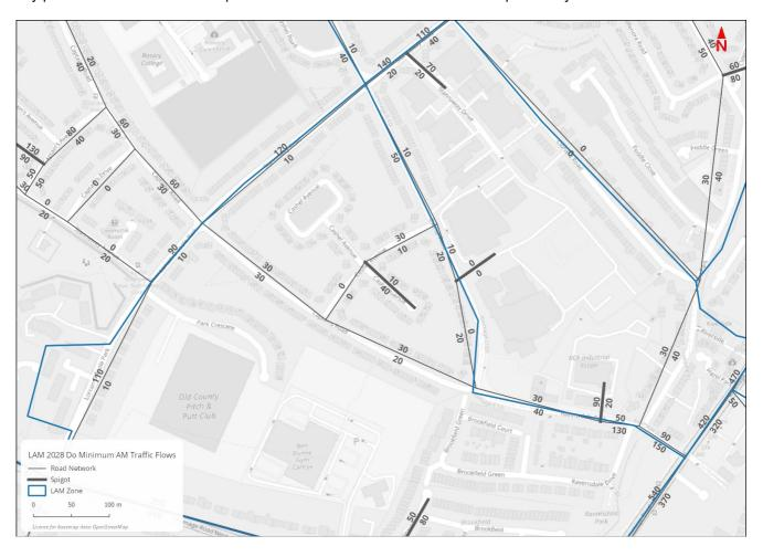
Diagram 5.8 Traffic zone boundaries and modelled road network with access points (spigots)
