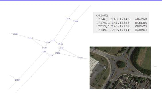
Diagram 5.3 Bus Connects LAM Node Matching (Junction C01-02)
