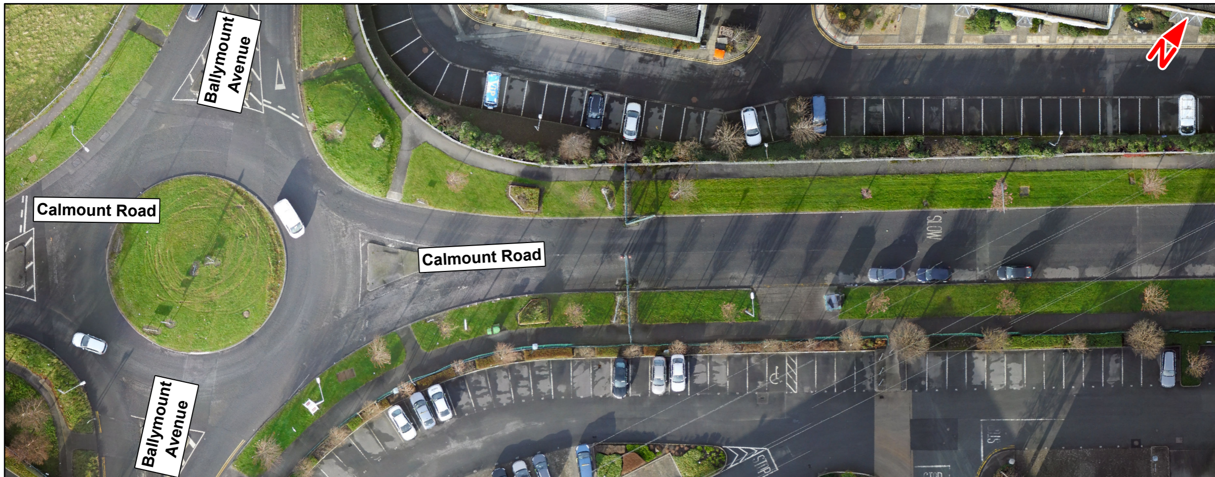
A) BALMOUNT AVENUE/ CALMOUNT ROAD FOUR-ARM ROUNDABOUT
